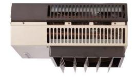
The Heavy Duty Unit Heater can be installed horizontally at high level to act as combination heater and destratification fan and operate as an Energy Saving Unit Heater. The directional louvres can be adjusted for optimum airflow. Hot air generated by heaters, process heat and machinery is automatically recycled from high level down to the occupied space. If the required low level temperature is still not attained, the heater elements are energised until this is the case.
