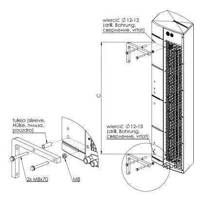
It is important to note that the minimum distance between the unit and the floor for installation with engine at the bottom is not less than 100mm. This allows access to the electrical terminal strip and to the water exchanger vent.
