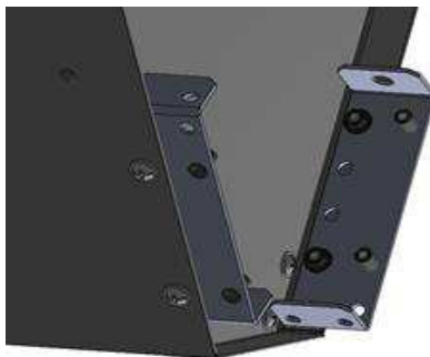
Installation of connector inside the curtain
