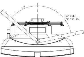
Use flexible connections to allow the heater to be turned to the sides. Depending on the flexible connections, the maximum turn is 78° - HEATER R1, R2, R3, 68° - HEATER ONE, to both sides. Figure shows maximum angle to one side and 50° to the other with minimal distance left for connections.
