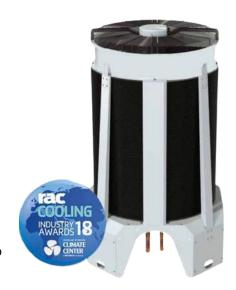
A single module can dissipate up to 61kW heat (at ambient air 25 °C; water-in 35°C & water-out 30°C) with a total footprint of only 1.21 m2.
